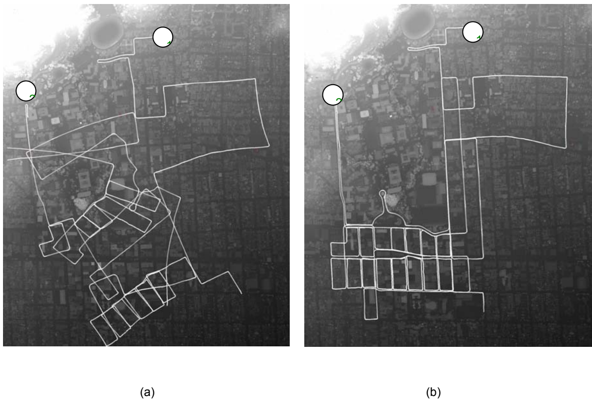
Figure 15.11: Driven paths superimposed on top of the DSM (a) before correction, and (b) after correction. The circles denote the starting position for paths 1 and 2, respectively.
