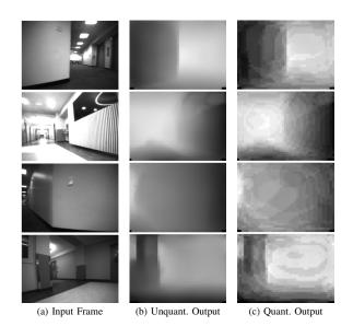
Fig. 6: Visualizations of our SIDE's model's performance on unseen test images. Frames were sourced from various local indoor hallway experiment environments.
