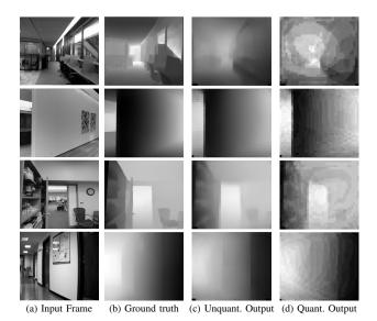
Fig. 5: Various examples of SIDE on images from our aggregated datasets. Top-Down: NYUv2, Matterport3D, Stanford 2D-3D, ICL-NUIMS. Ground-truth for Matterport3D, Stanford 2D-3D, ICL-NUIMS generated via DPT-Large.
