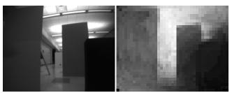
(a) Camera grayscale input frame (b) Computed inference depth map
