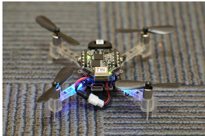
Fig. 1: The Bitcraze Crazyflie 2.1 facing away from the camera with the AI Deck and Flow Deck v2 attached.
