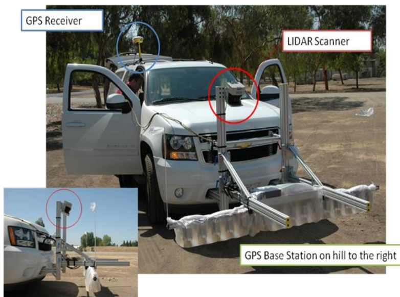
Figure 1: Data acquisition vehicle with the LiDAR scanner and GPS receiver.
