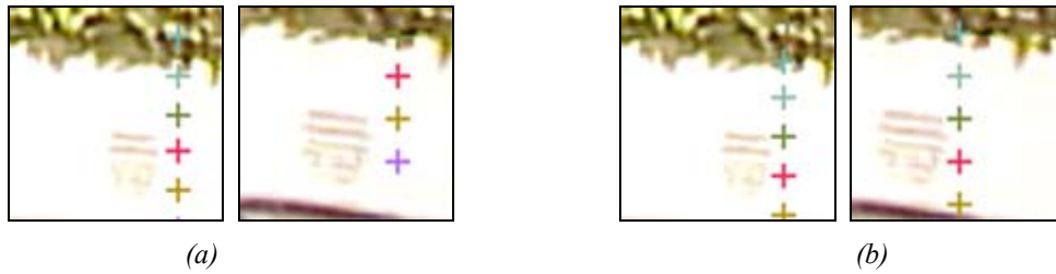
Figure 12: Reprojections of model points in the images. (a) The left images show the reprojections of selected model points in two images with the original rough pose estimation. Projections of the same 3D point are drawn in the same colour in both images. The original pose is clearly incorrect. (b) The right images show the same points projected with the new pose, found using the proposed algorithm. The images clearly match the model well.
