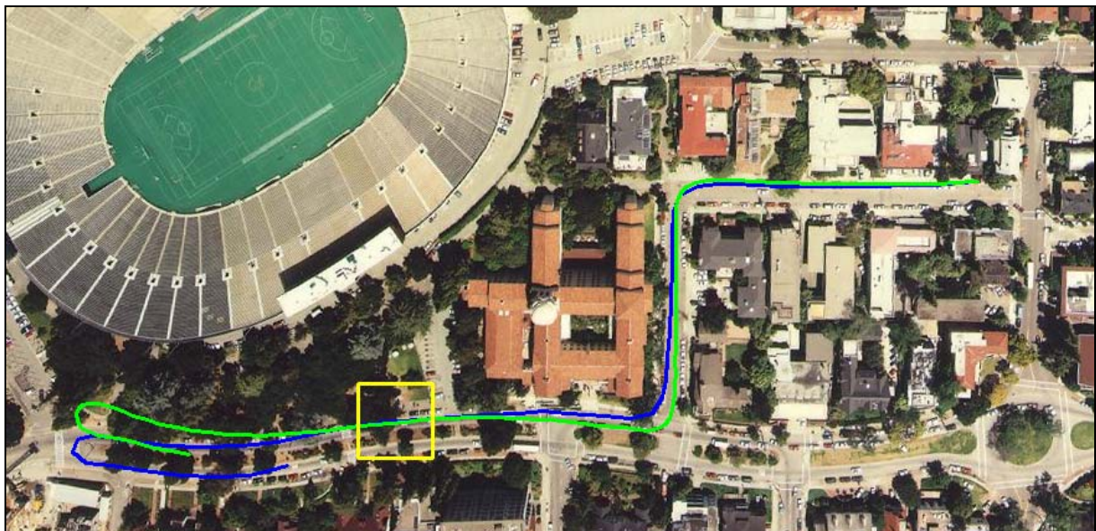
Figure 18: The Ihouse sequence: Plot of computed vehicle motion in the ground plane, computed using no initial transformations, overlaid on an aerial photo of the area. The path obtained using no initial transformations is shown in green, the path obtained using laser scan-matching as initialisation is shown in blue. The main error seems to occur in the highlighted area shown.
