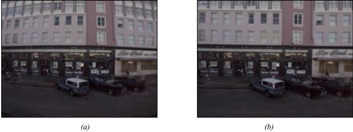
Figure 6: The results of camera calibration. The image in (a) shows significant radial distortion. (b) shows the same image after the radial distortion has been removed, using the estimated parameters.
