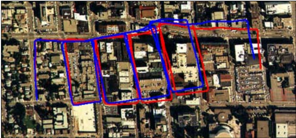
Figure 16: The downtown sequence: Plots of vehicle motion in the ground plan, overlaid on an aerial photo of the area. No colour photo was available. The original path obtained from laser scan matching is shown in red, the path obtained using our algorithm is shown in blue. A gross error occurs at the highlighted region, for reasons discussed below.
