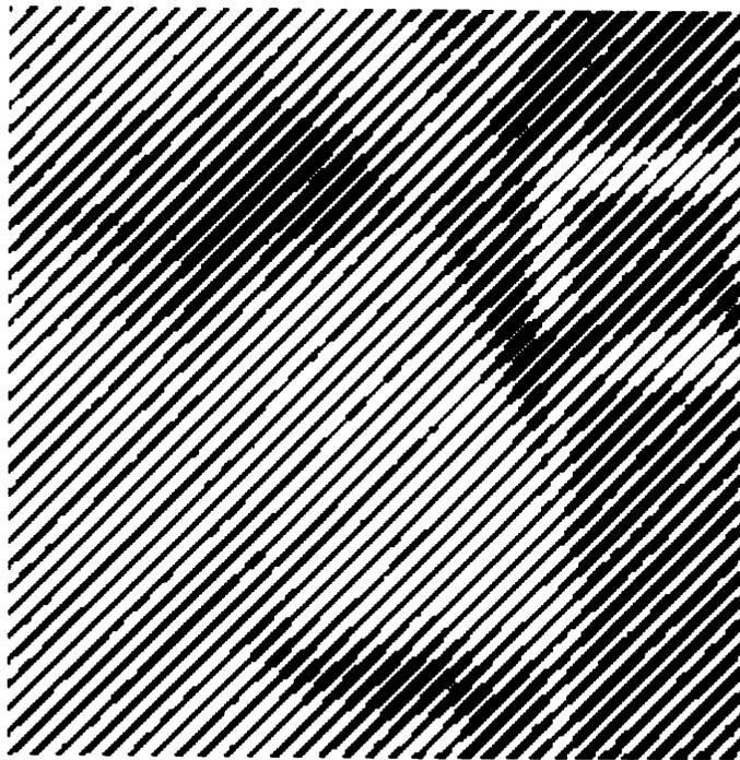
Figure 3.7: *One bit amplitude quantized version of the sum of the original cman picture and  $128(1 + \cos(2\pi(32x + 32y)))$ .*
