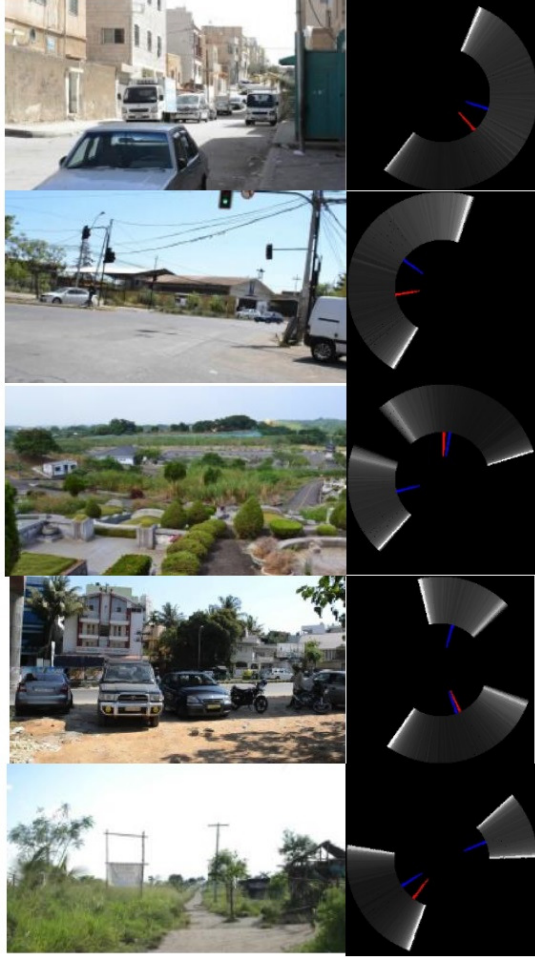
Fig. 6. A sampling of success cases; the blue marks indicate means of distributions; the red, ground truth headings.
