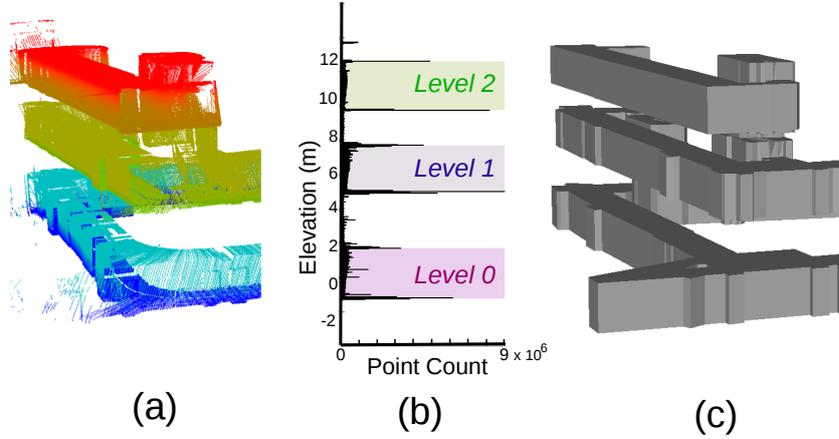
**Fig. 2.** An example point-cloud partitioning by height: (a) the input point-cloud, showing geometry for three levels; (b) the vertical histogram showing estimates of each building level height; (c) the produced mesh of this building scan.
