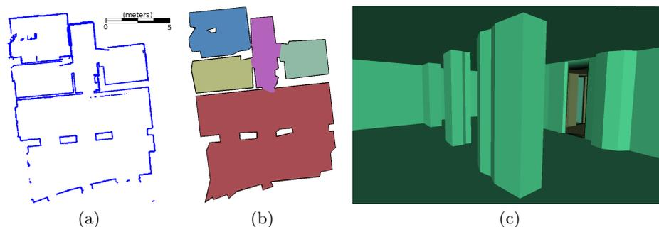
**Fig. 9.** Apartment complex office: (a) Input represented by 3,462 wall samples; (b) generates floor plan with 5 rooms; (c) extruded 3D mesh represented with 512 triangles. Total processing time required is 1.2 seconds.
