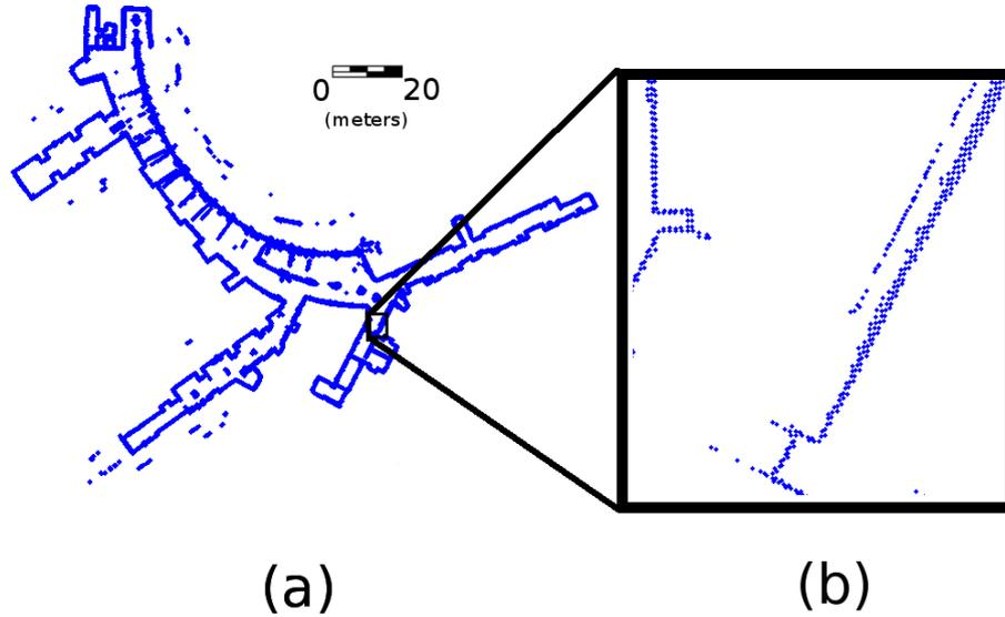
**Fig. 1.** Example input wall samples of hotel hallways and lobby generated from a particle filter system. (a) Wall samples of full model; (b) close up of wall in model.
