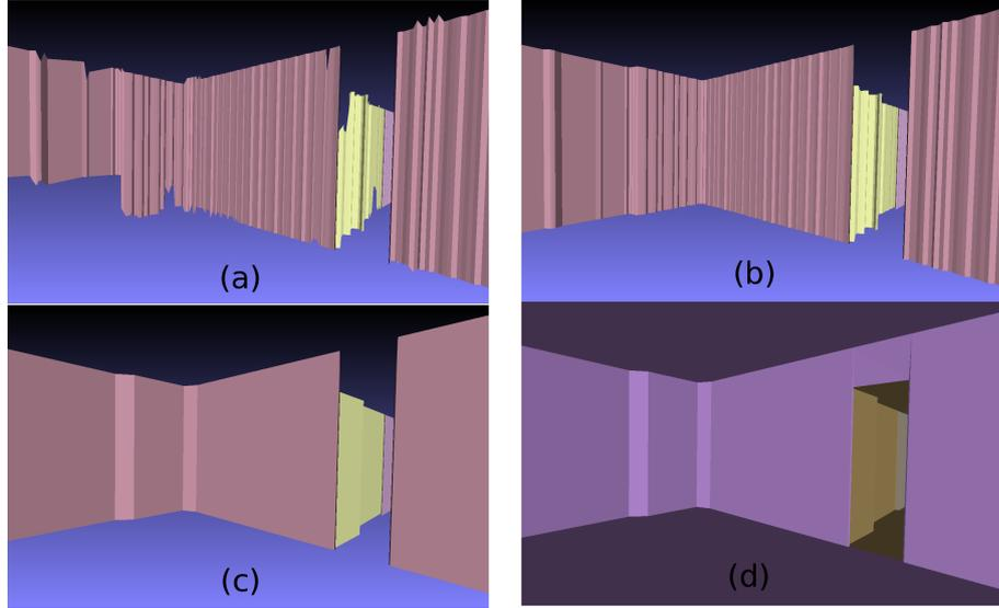
**Fig. 6.** Example of creating a 3D extruded mesh from 2D wall samples: (a) walls of generated floor plan with estimated height ranges; (b) floor and ceiling heights are grouped by room; (c) simplification performed on walls; (d) floor and ceiling triangles added to create a watertight mesh.
