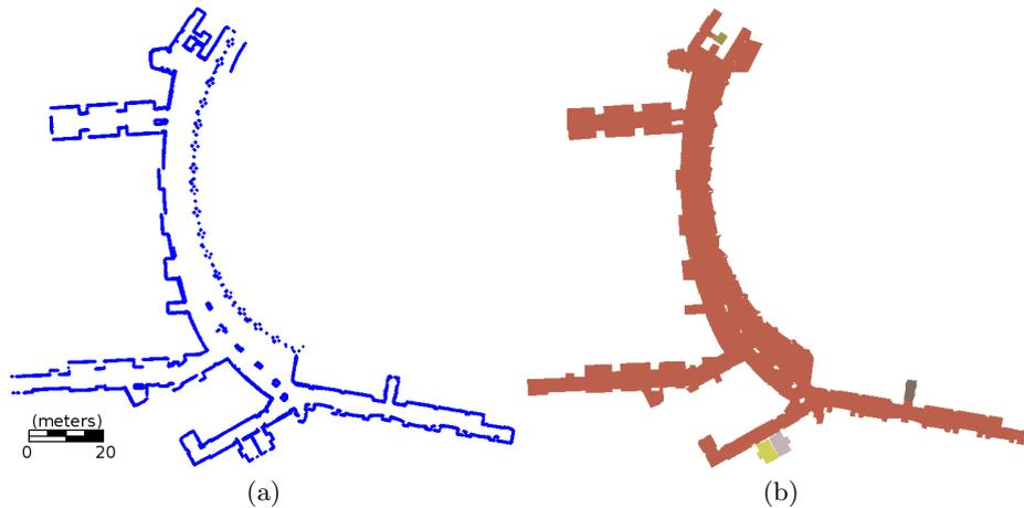
**Fig. 10.** Hotel lobby and hallways: (a) Input represented by 33,582 wall samples; (b) generates floor plan with 5 rooms. Extruded 3D mesh represented with 5,012 triangles. Total processing time required is 8.5 seconds.
