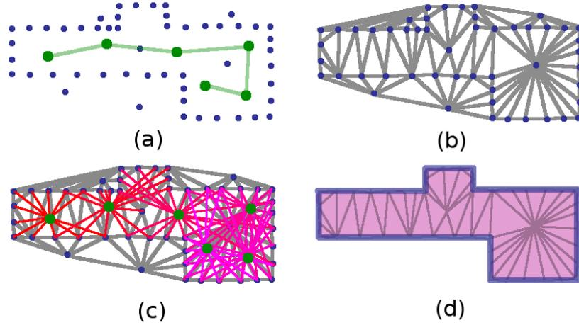
**Fig. 3.** Example of carving process to find interior triangles: (a) wall samples (in blue) with path of scanner (in green); (b) Delaunay Triangulation of wall samples; (c) laser scans from each pose (in red); (d) triangles that intersect with laser scans (in pink), used as interior triangles, with building model border (in blue).
