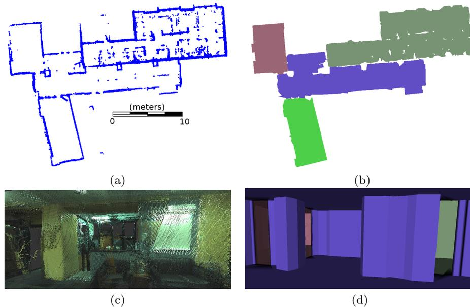
**Fig. 11.** University office area: (a) Input represented by 12,183 wall samples; (b) generates floor plan with 4 rooms; (c) original point-cloud of scanned area; (d) extruded 3D mesh represented with 4,912 triangles. Processing time required to convert wall samples to mesh is 7 seconds.
