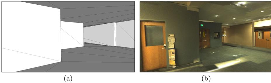
**Fig. 8.** Interior view of 3D extruded reconstructed model: (a) without and (b) with texture-mapping [5].
