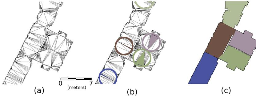
**Fig. 4.** Example room seed partitioning: (a) interior triangulation; (b) the room seed triangles, and their corresponding circumcircles; (c) room labels propagated to all other triangles.
