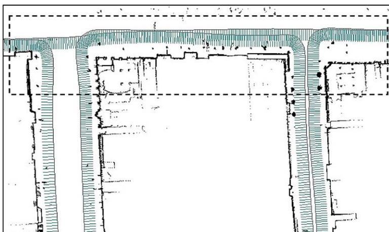
*Figure 18.* Horizontal scan points of the corrected path. Scan points are drawn in black and the driven path with the direction of the vertical laser scanner is marked in gray. The area inside the dashed rectangle has been passed and scanned multiple times. The scan points inside buildings correspond to interior walls scanned through the windows.
