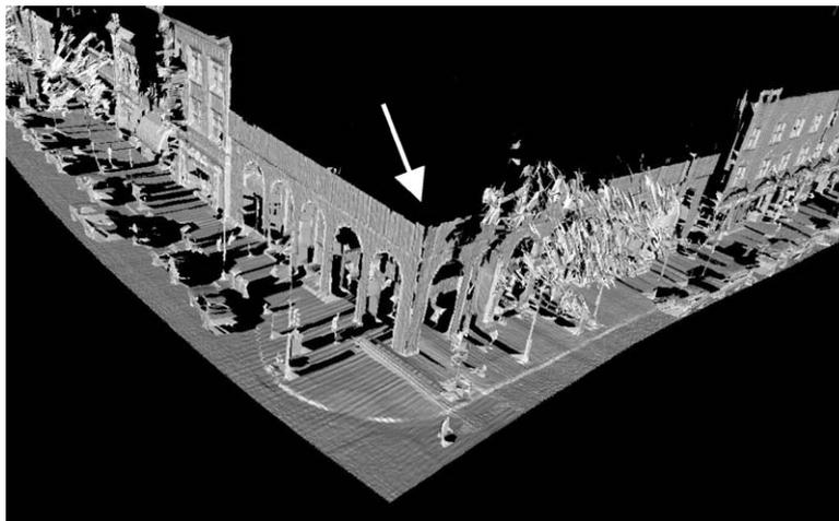
*Figure 22.* Alignment of two independently acquired facades.
