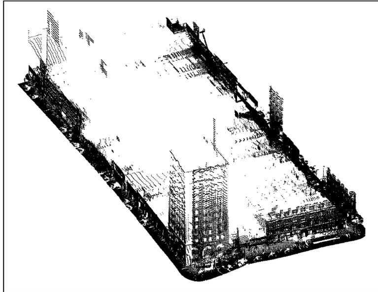
Figure 19. Structured point cloud for a city block.
