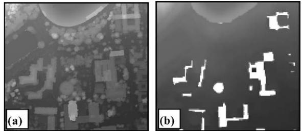
Figure 9. DTM computation: (a) Original DSM, (b) estimated DTM, with blank spots remaining at building locations.
