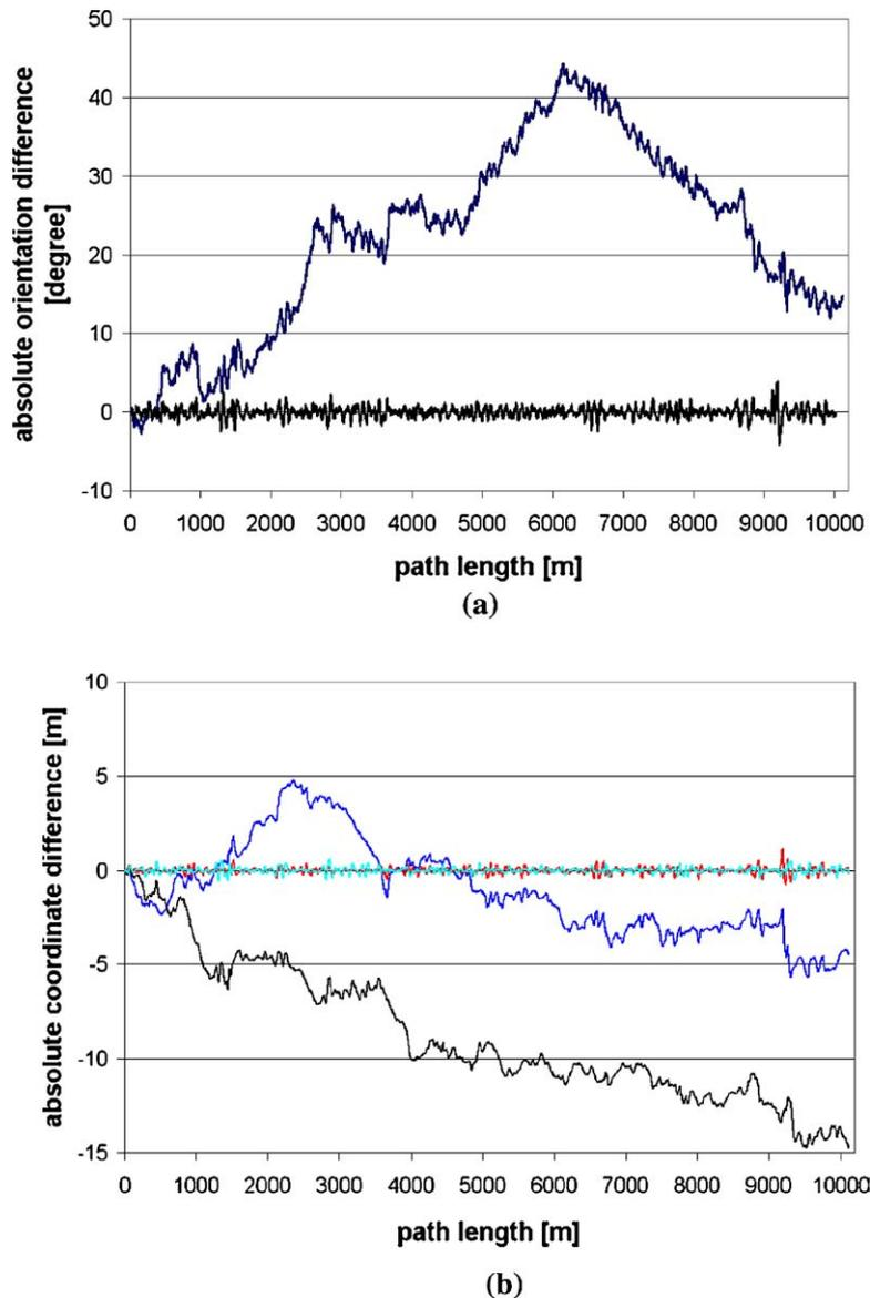
*Figure 14.* Global correction along the traveled path: (a) yaw angle difference between initial pose and intermediate pose before and after correction, (b) differences of  $x$  and  $y$  coordinates between angle-corrected pose and intermediate pose, before and after correction. In both diagrams, the differences after corrections are the curves close to the horizontal axis.
