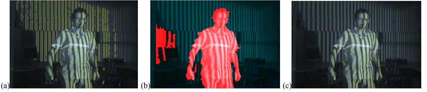
Figure 5: (a) Detected V-lines; (b) Detected IR foreground silhouette shown in red; (c) V-lines clipped to the foreground silhouette.
