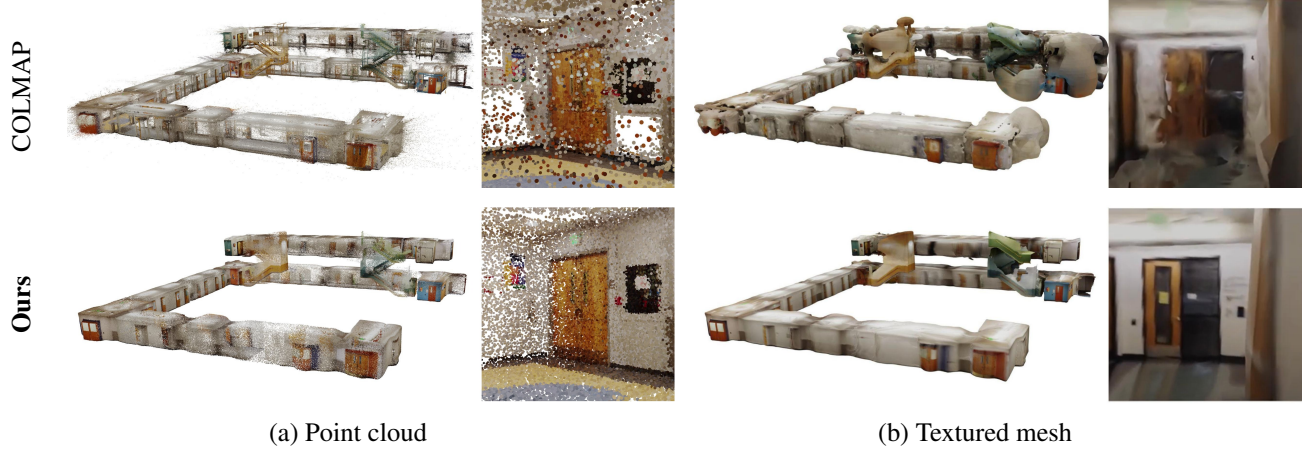
Figure 3: Qualitative results of our reconstruction results. (a) Our dense point cloud is dense on low-textured areas and is far less noisy than COLMAP. (b) Our method reconstructs more accurate textured mesh and is more robust than COLMAP on reflective and low-textured surface.
