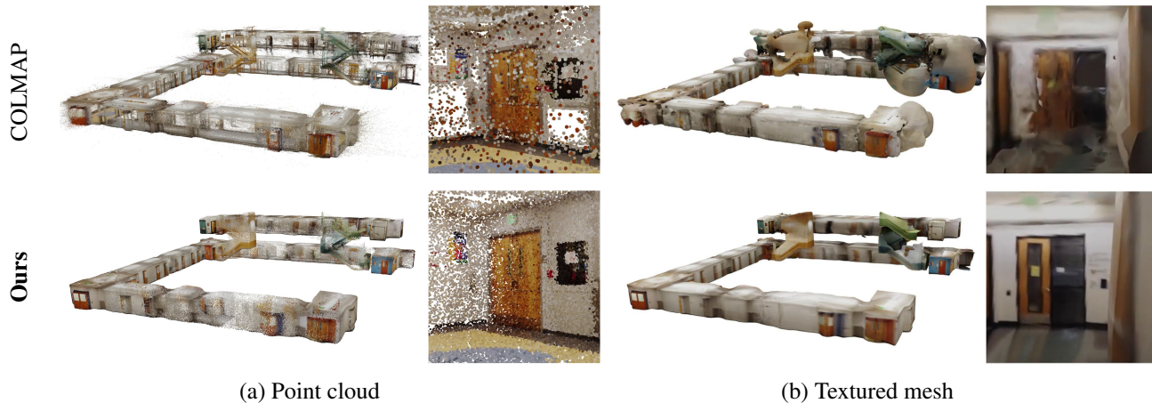
Figure 3: Qualitative results of our reconstruction results. (a) Our dense point cloud is dense on low-textured areas and is far less noisy than COLMAP. (b) Our method reconstructs more accurate textured mesh and is more robust than COLMAP on reflective and low-textured surface.
