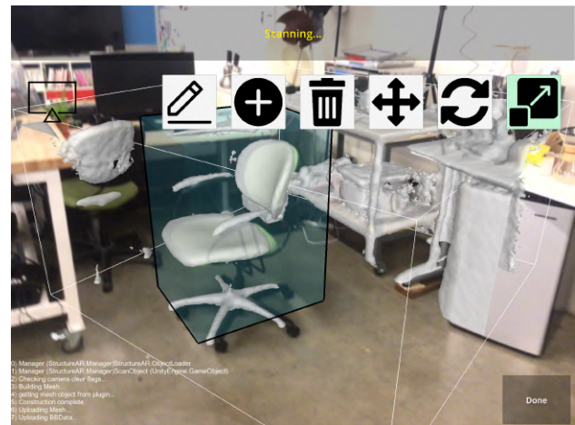
Figure 3: Screenshot of the application in action: A scanned mesh, shown in white, is superimposed on top of camera feed in real-time. A bounding box, shown in translucent blue, has been placed around the chair.
