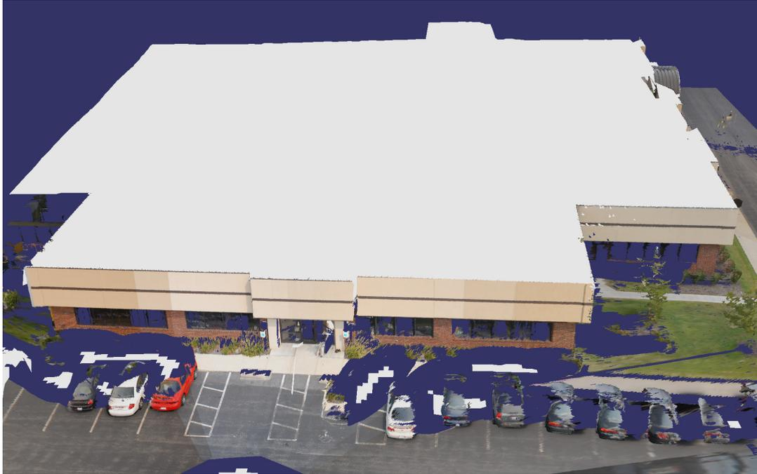
**Figure 11. A merged model, with vertices from airborne data colored white.**
