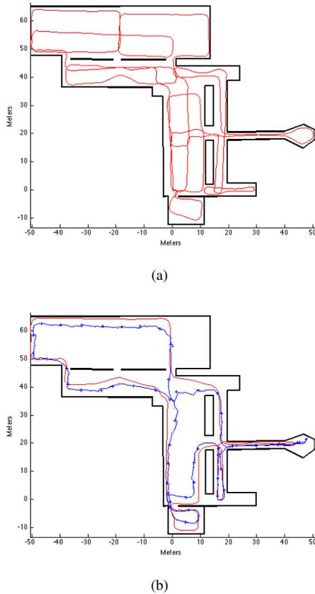
Fig. 3. Example test paths in Doe Library. Red is the "ground truth" as measured by the foot mounted IMU. Blue is the path estimated by our system. 'x's indicate locations where a WiFi update is received. (a) Database collection path, (b) Path D2 from Nexus 5
