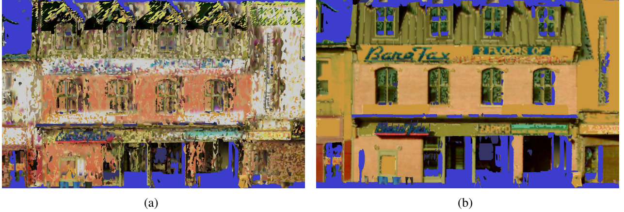
Figure 10: Mesh (a) with redundant surfaces and (b) without redundant surfaces. The point clouds used to generate these meshes are not from S1 or S2. Instead, they are from a dataset which was obtained using multiple sensor passes.
