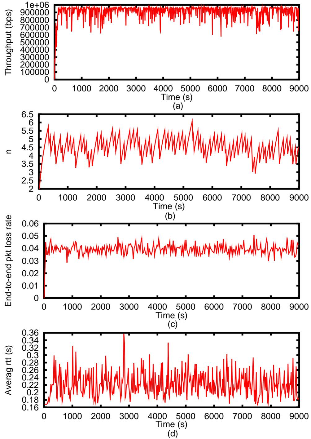
Figure 5.26. NS-2 simulations of E-AIOTFRC for  $B_w = 1Mbps$  and  $p_w = 0.04$ ; (a)throughput, (b) number of connections , (c) end-to-end packet loss rate, (d) end-to-end RTT, all as a function of time.
