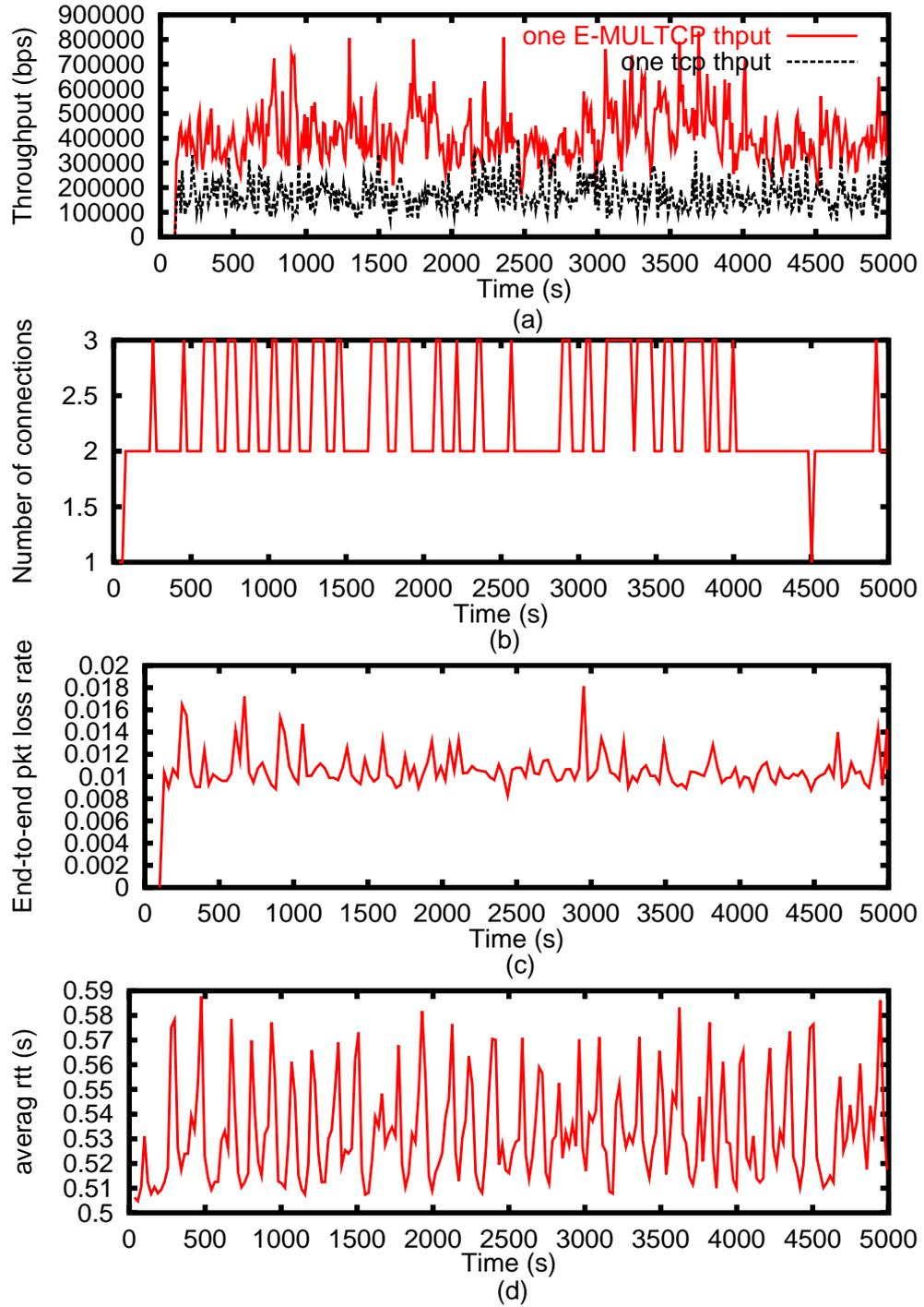
Figure 5.8. NS-2 simulation results for the case  $p_w = 0.01, \gamma = 0.1$  for E-MULTTCP+TCP scenario: (a) throughput, (b) number of connections, (c) end-to-end packet loss rate, (d) end-to-end RTT, all as a function of time.
