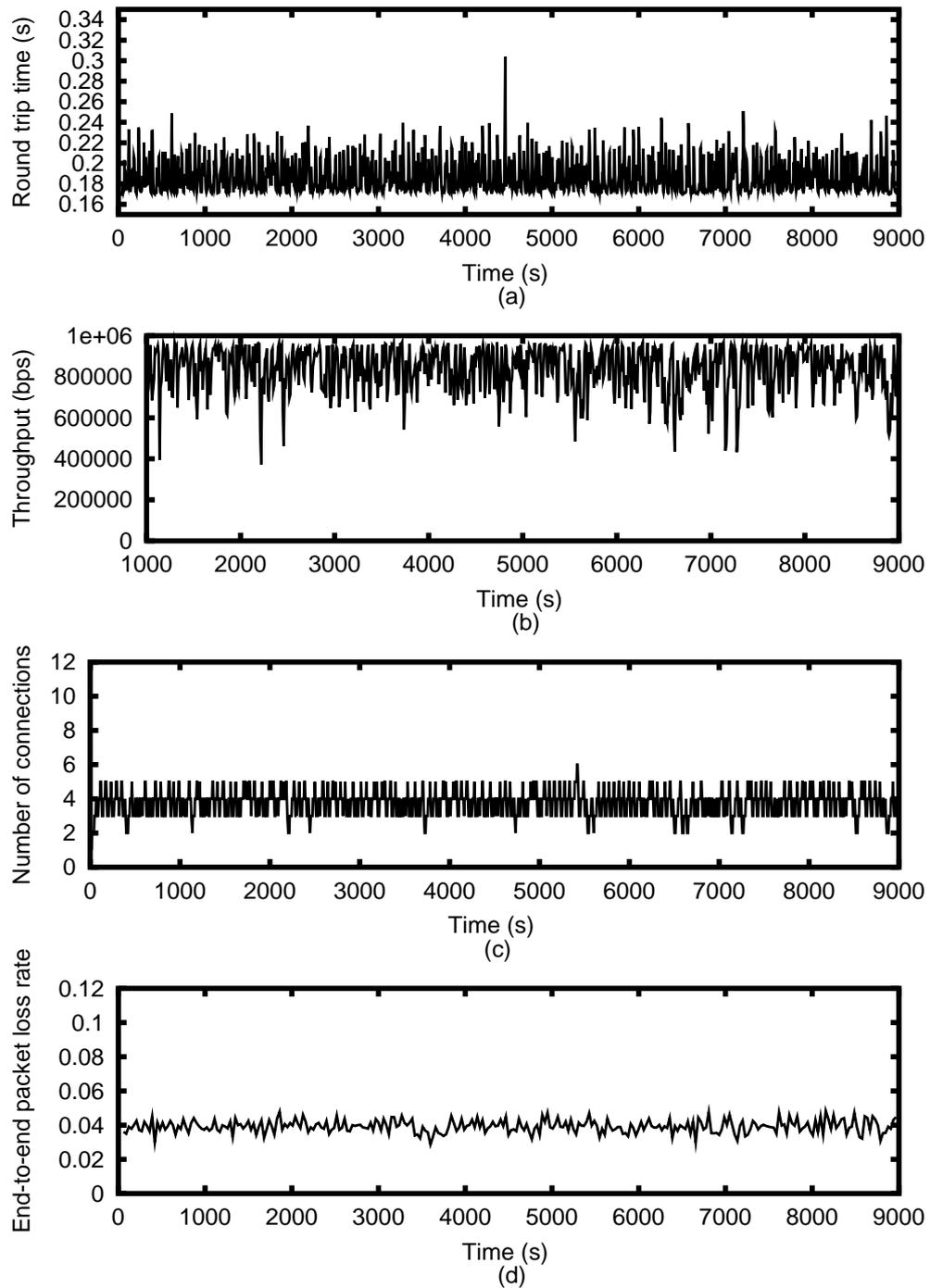
Figure 5.23. NS-2 simulations of MULTFRC for  $B_w = 1Mbps$  and  $p_w = 0.04$ ; (a) end-to-end round trip time, (b) throughput, (c) end-to-end packet loss rate, (d) number of connections, all as a function of time.
