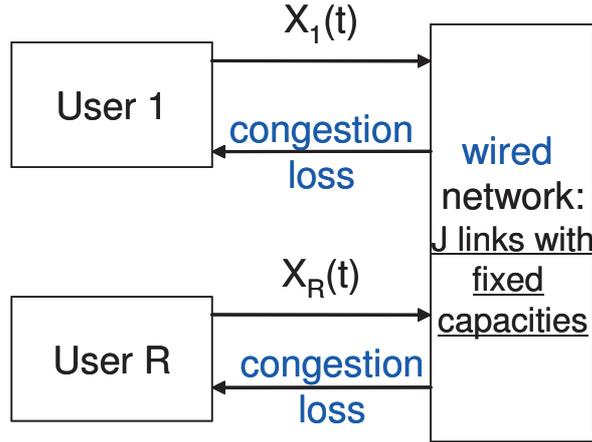
Figure 3.1. Feedback control modeling: TCP over wired networks
