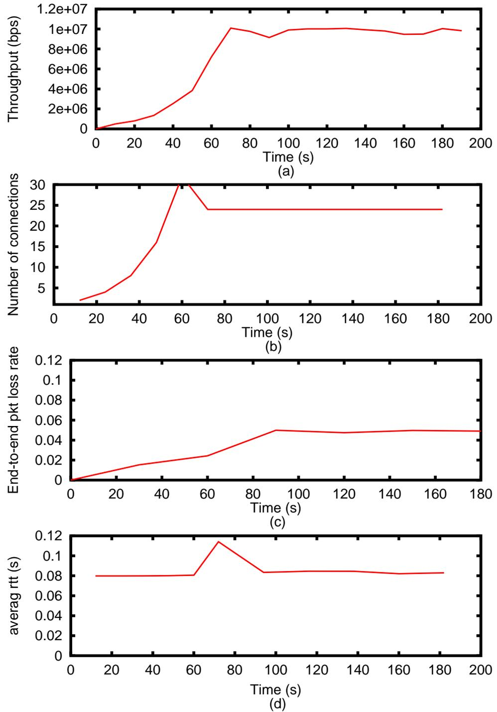
Figure 5.9. NS-2 simulation results for the case  $p_w = 0.05$  for E-MULTTCP with slow start: (a) throughput, (b) number of connections, (c) end-to-end packet loss rate, (d) end-to-end RTT, all as a function of time.
