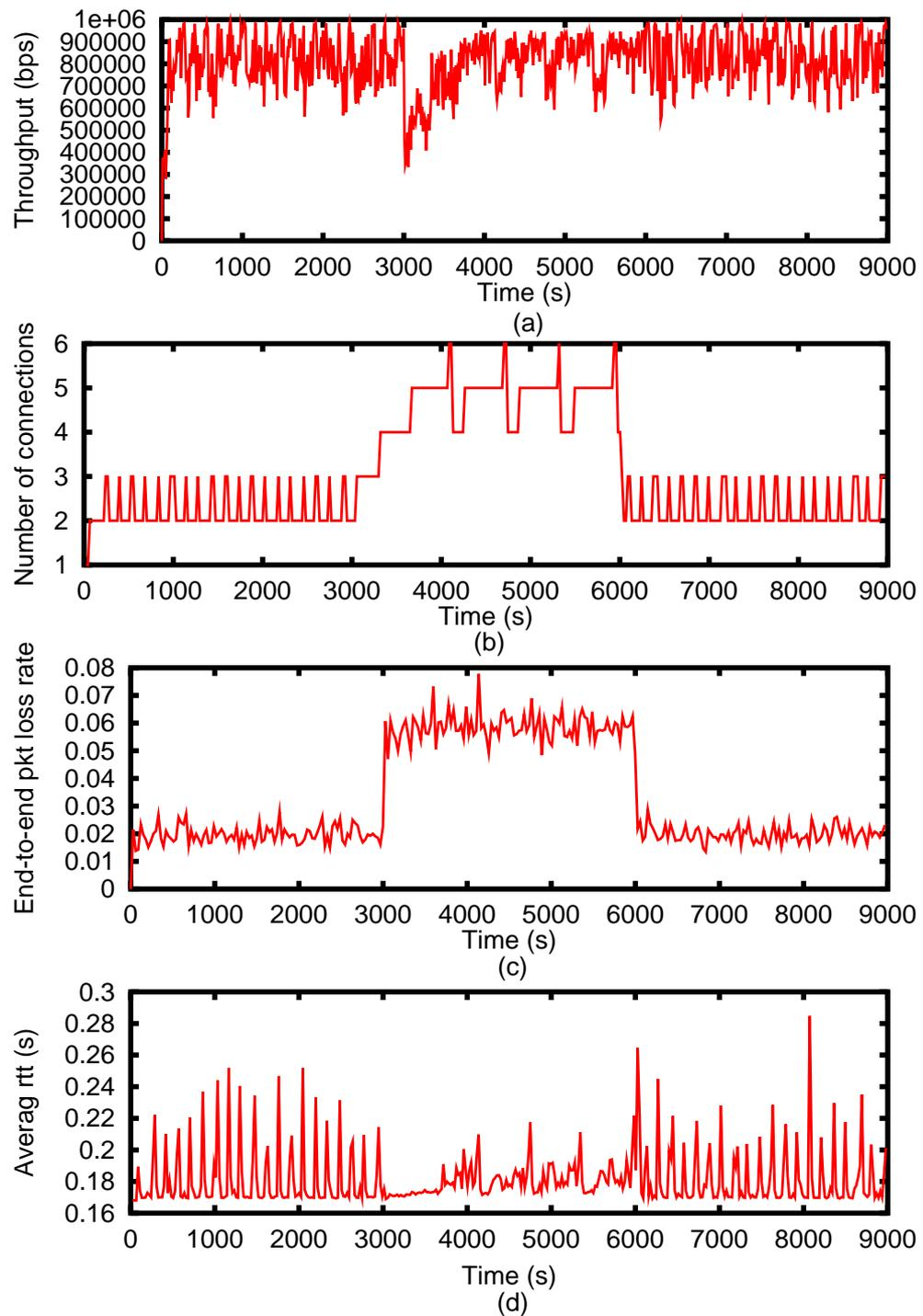
Figure 5.12. NS-2 simulation results of E-MULTFRC as  $p_w$  changes from 0.02 to 0.06 and back again; (a) end-to-end round trip time, (b) throughput, (c) numbers of connections, (d) end-to-end packet loss rate, all as a function of time.
