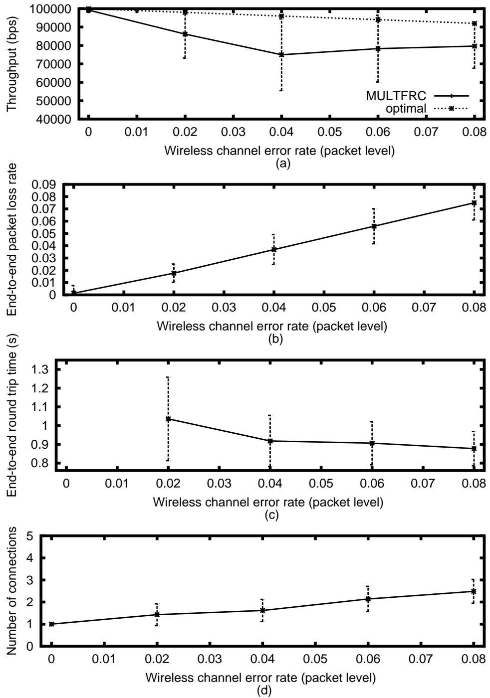
Figure 5.22. NS-2 simulations of MULTFRC for  $B_w = 100 \text{ kbps}$  and  $RTT_{min} = 757 \text{ ms}$ ; (a) throughput, (b) end-to-end packet loss rate, (c) end-to-end round trip time, (d) number of connections, all as a function of packet level wireless channel error rate.
