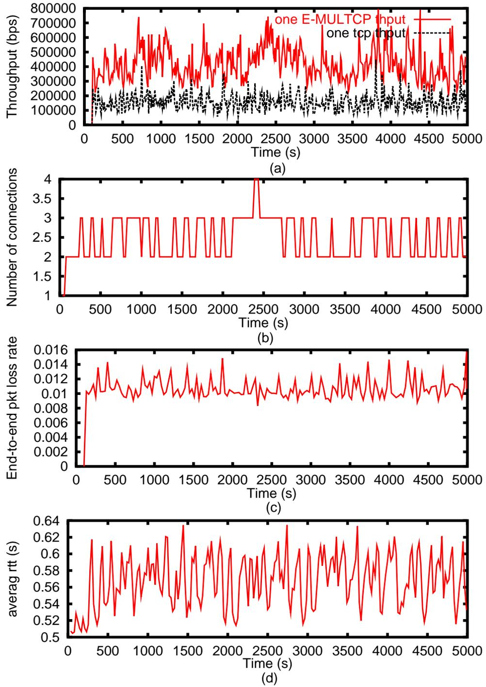
Figure 5.7. NS-2 simulation results for the case  $p_w = 0.01, \gamma = 0.2$  for E-MULTCP+TCP scenario: the dynamics of (a) throughput, (b) number of connections, (c) end-to-end packet loss rate, (d) end-to-end RTT, all as a function of time.
