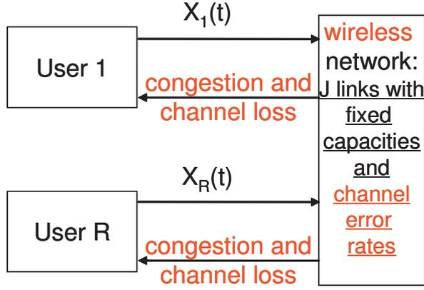
Figure 3.2. Feedback control modeling: TCP over wireless networks
