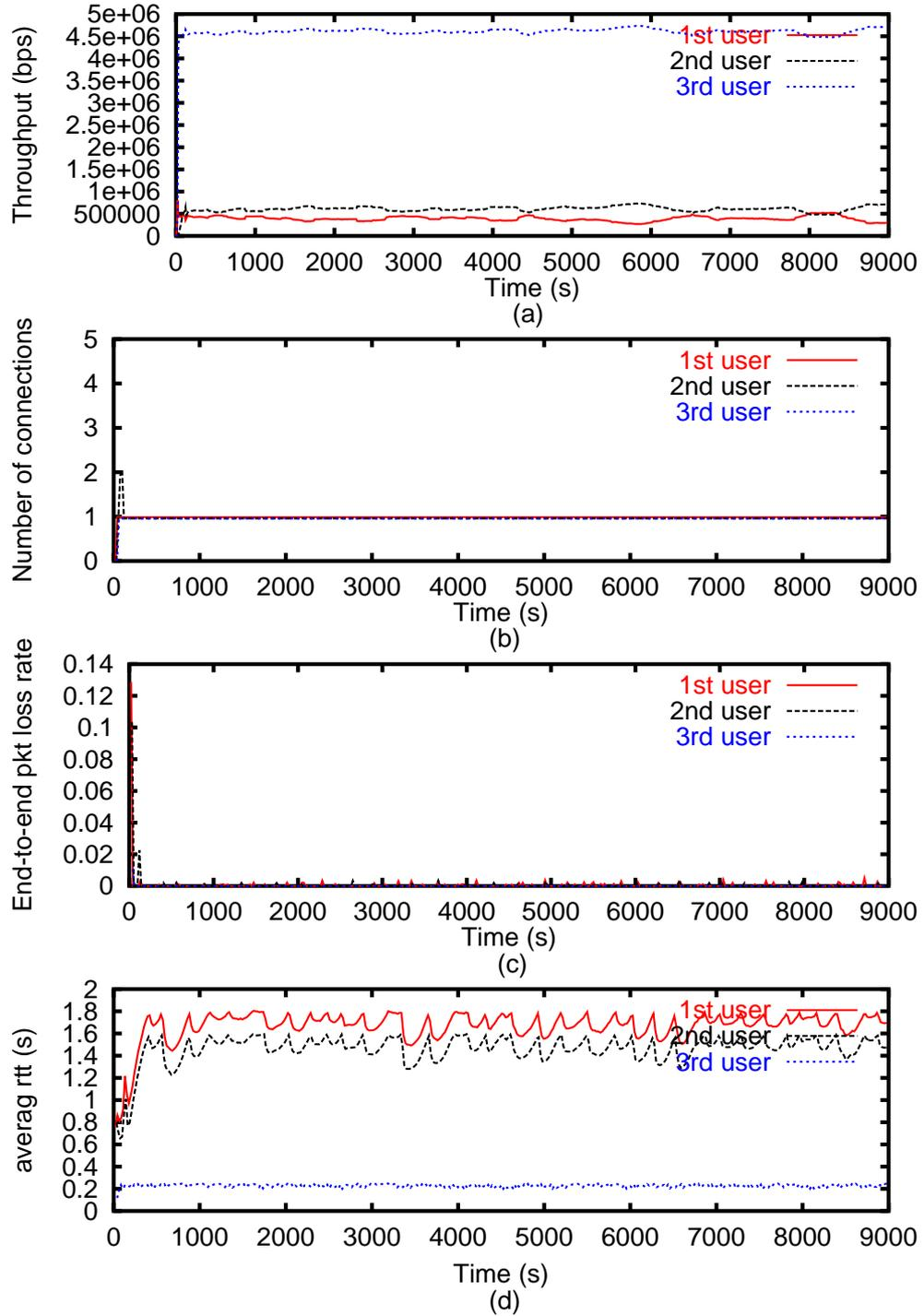
Figure 5.16. NS-2 simulations of E-MULTFRC for the topology shown in Figure 5.13 with  $p_w^1 = 0.00, p_w^2 = 0.00$ : (a) throughput, (b) number of connections, (c) end-to-end packet loss rate and (d) average *rtt*.
