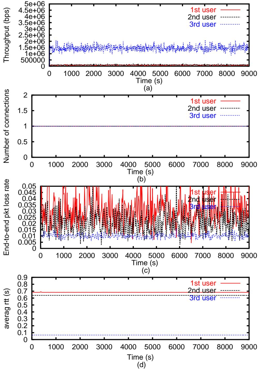
Figure 5.14. NS-2 simulations of one TFRC for the topology shown in Figure 5.13 with  $p_w^1 = 0.02, p_w^2 = 0.01$ : (a) throughput, (b) number of connections, (c) end-to-end packet loss rate and (d) average *rtt*.
