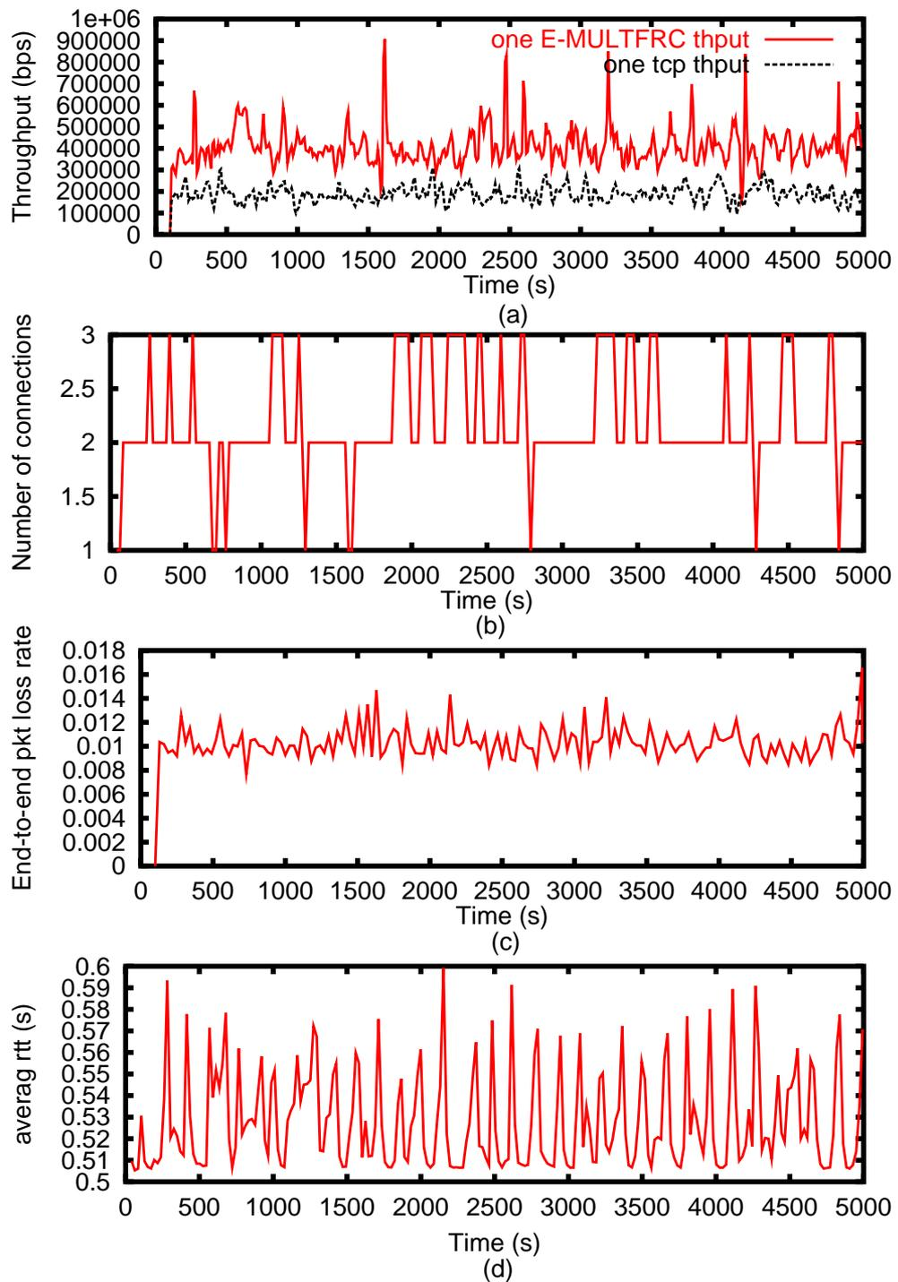
Figure 5.18. NS-2 simulation results of E-MULTFRC for the case  $p_w = 0.01, \gamma = 0.1$  for E-MULTFRC+TCP scenario: (a)throughput, (b) number of connections , (c) end-to-end packet loss rate, (d) end-to-end RTT, all as a function of time.
