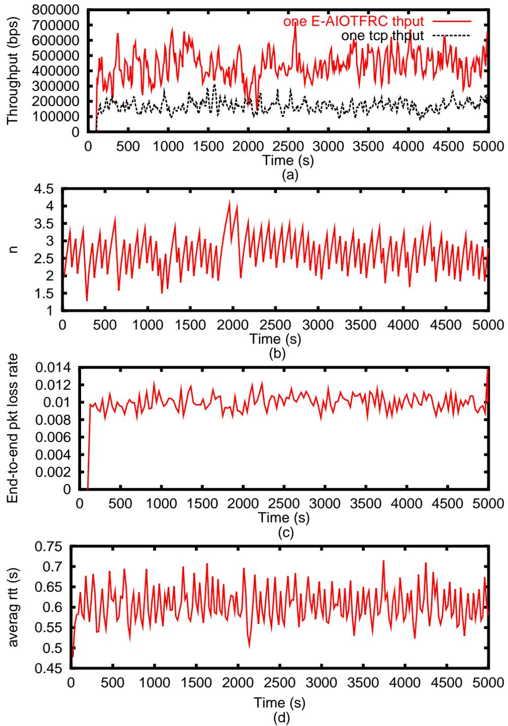
Figure 5.27. NS-2 simulation results of E-AIOTFRC coexisting with TCP, for the case  $p_w = 0.01, \gamma = 0.5$ : the dynamics of (a) throughput, (b) number of connections, (c) end-to-end packet loss rate, (d) end-to-end RTT, all as a function of time.
