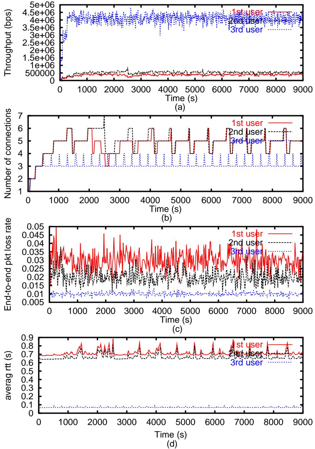
Figure 5.15. NS-2 simulations of E-MULTFRC for the topology shown in Figure 5.13 with  $p_w^1 = 0.02, p_w^2 = 0.01$ : (a) throughput, (b) number of connections, (c) end-to-end packet loss rate and (d) average *rtt*.
