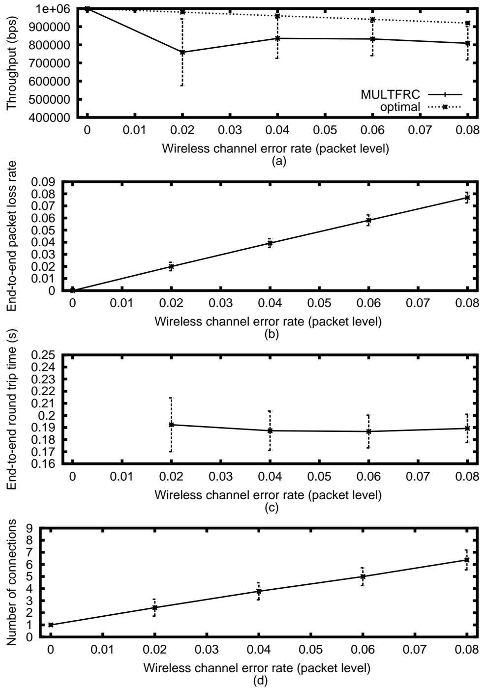
Figure 5.21. NS-2 simulations of MULTFRC for  $B_w = 1 \text{ Mbps}$  and  $RTT_{min} = 168 \text{ ms}$ ; (a) throughput, (b) end-to-end packet loss rate, (c) end-to-end round trip time, (d) number of connections, all as a function of packet level wireless channel error rate.
