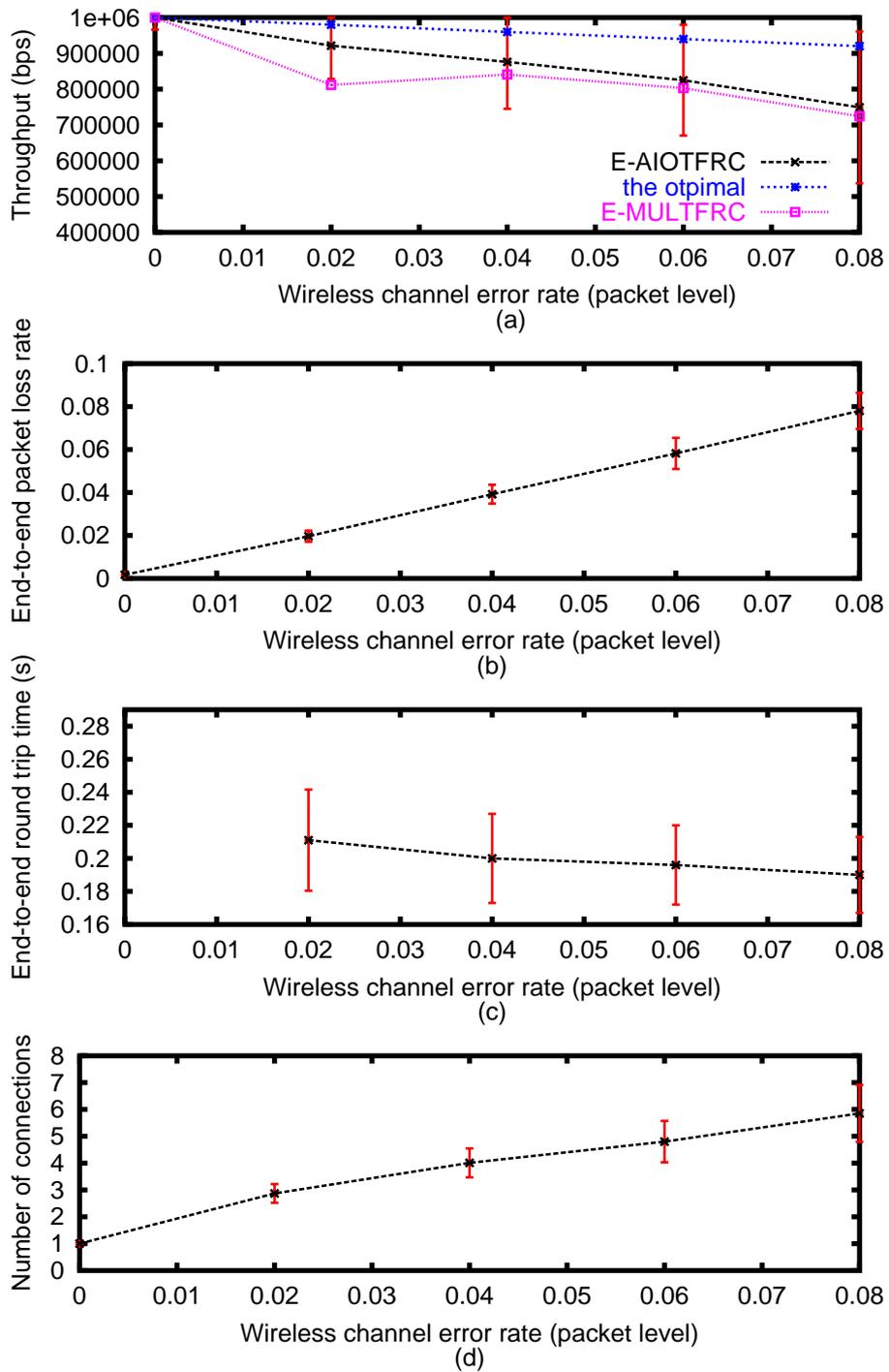
Figure 5.25. NS-2 simulations of E-AIOTFRC for Bw = 1 Mbps and RTT<sub>min</sub> = 168 ms; (a) throughput, (b) end-to-end packet loss rate, (c) end-to-end RTT, (d) number of connections, all as a function of packet error rate on the wireless channel.
