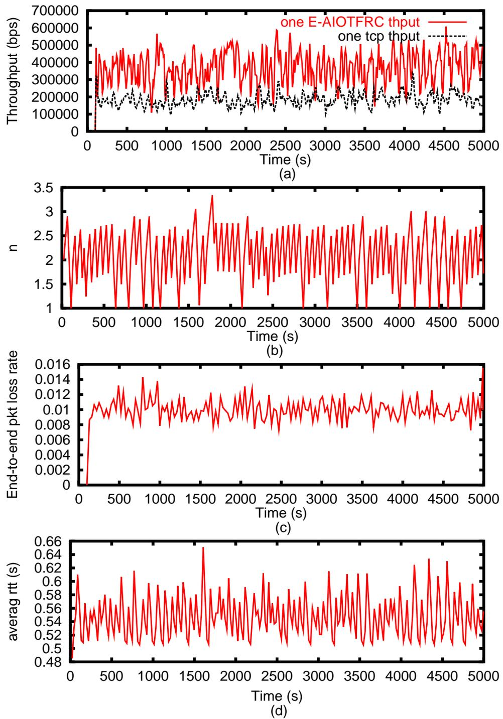
Figure 5.28. NS-2 simulation results of E-AIOTFRC coexisting with TCP, for the case  $p_w = 0.01, \gamma = 0.1$ : (a)throughput, (b) number of connections , (c) end-to-end packet loss rate, (d) end-to-end RTT, all as a function of time.
