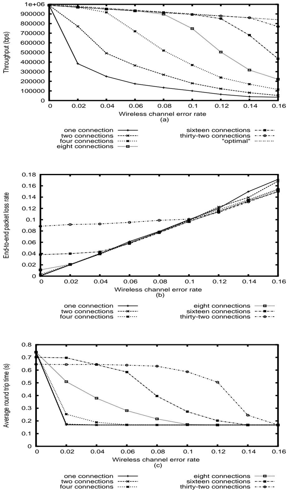
Figure 2.4. NS-2 simulations of the simple case study: (a) End-to-end throughput, (b) packet loss rate, and (c) round trip time as a function of wireless channel error rate,  $p_w$ , for different number of connections.
