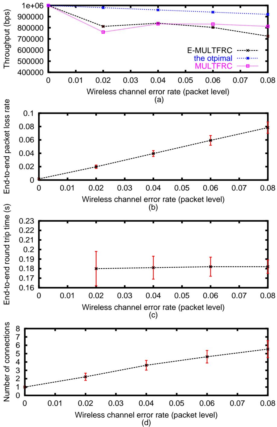
Figure 5.10. NS-2 simulations of E-MULTFRC for  $B_w = 1 \text{ Mbps}$  and  $RTT_{min} = 168 \text{ ms}$ ; (a) throughput, (b) end-to-end packet loss rate, (c) end-to-end round trip time, (d) number of connections, all as a function of packet level wireless channel error rate.
