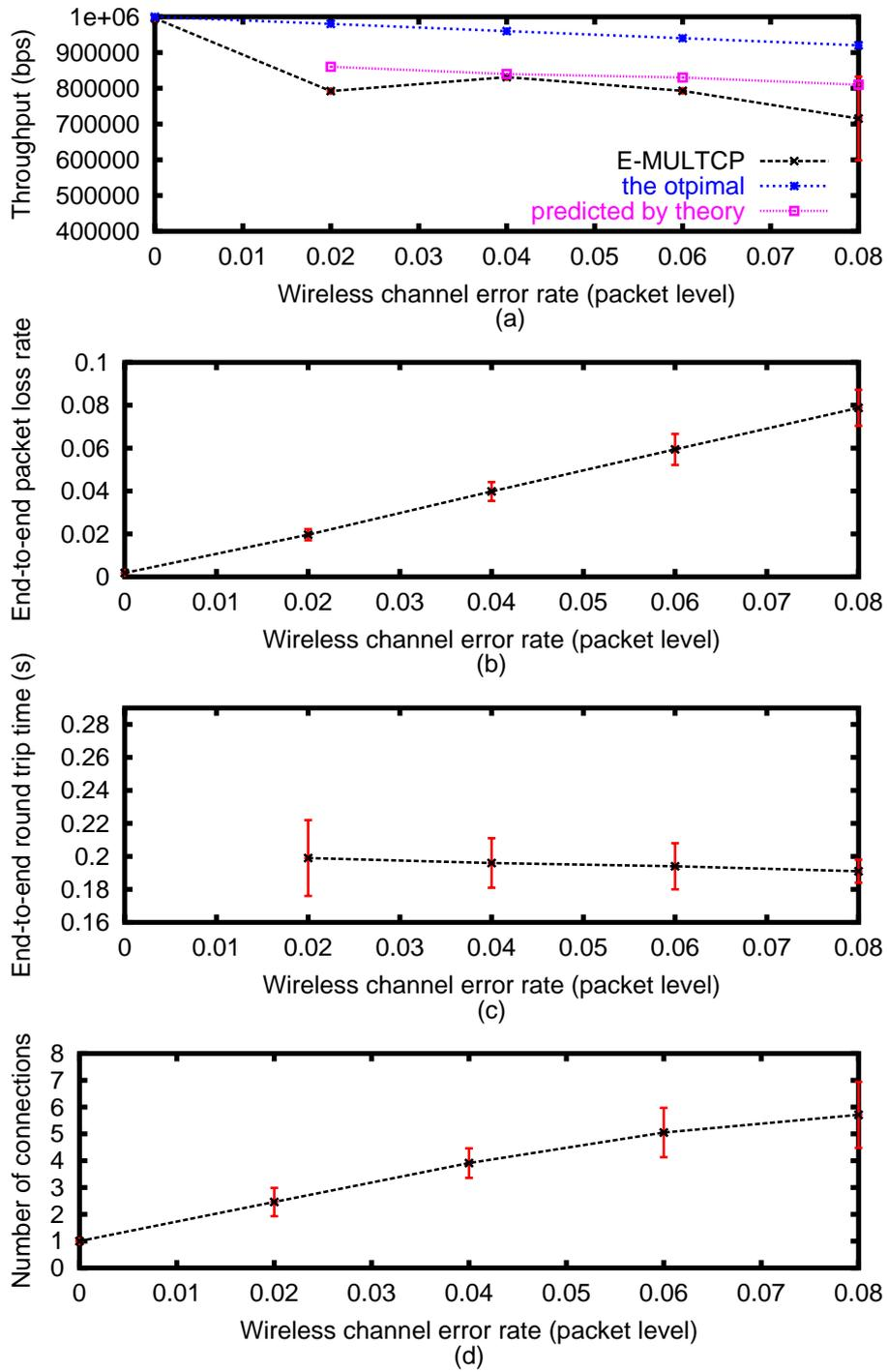
Figure 5.2. NS-2 simulations of E-MULTCP for  $B_w = 1 \text{ Mbps}$  and  $RTT_{min} = 168 \text{ ms}$ , for  $\beta = 0.75$ ; (a) throughput, (b) end-to-end packet loss rate, (c) end-to-end round trip time, (d) number of connections, all as a function of packet level wireless channel error rate.
