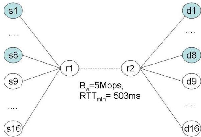
Figure 5.6. The simulation topology for E-MULTTCP's fairness evaluation.
