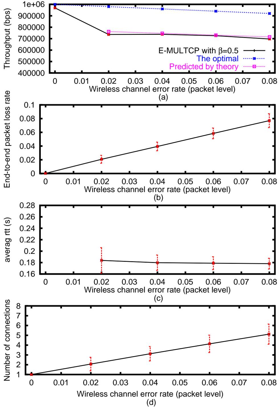
Figure 5.3. NS-2 simulations of E-MULTTCP for  $B_w = 1 \text{ Mbps}$  and  $RTT_{min} = 168 \text{ ms}$ , for  $\beta = 0.5$ ; (a) throughput, (b) end-to-end packet loss rate, (c) end-to-end round trip time, (d) number of connections, all as a function of packet level wireless channel error rate.
