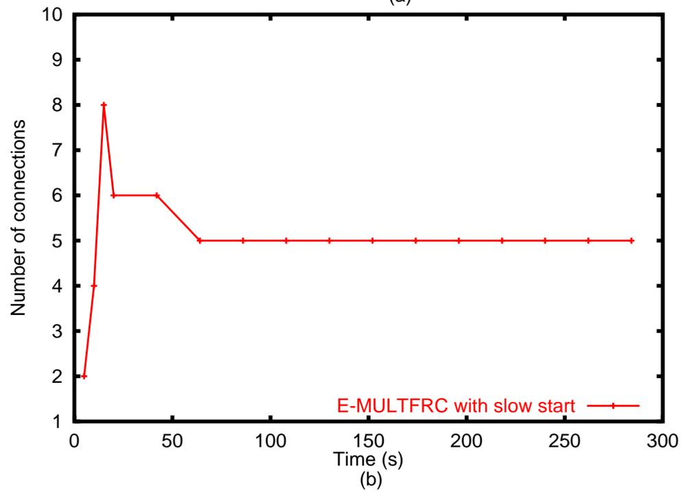
Figure 5.19. Performance comparison between E-MULTFRC and VTP, in the presence of random loss: (a) throughput; (b) the number of connections opened by E-MULTFRC.
