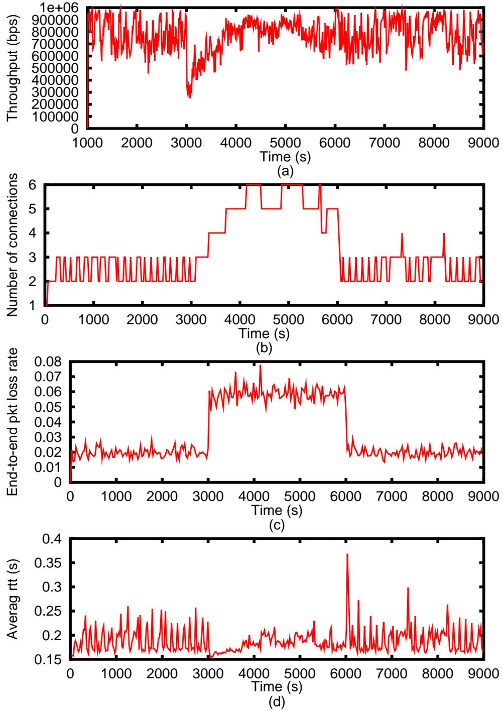
Figure 5.4. NS-2 simulation results of E-MULTTCP with  $\beta = 0.75$  as  $p_w$  changes from 0.02 to 0.06 and back again, for  $\alpha = 0.25$ ; (a) end-to-end round trip time, (b) throughput, (c) number of connections, (d) end-to-end packet loss rate, all as a function of time.
