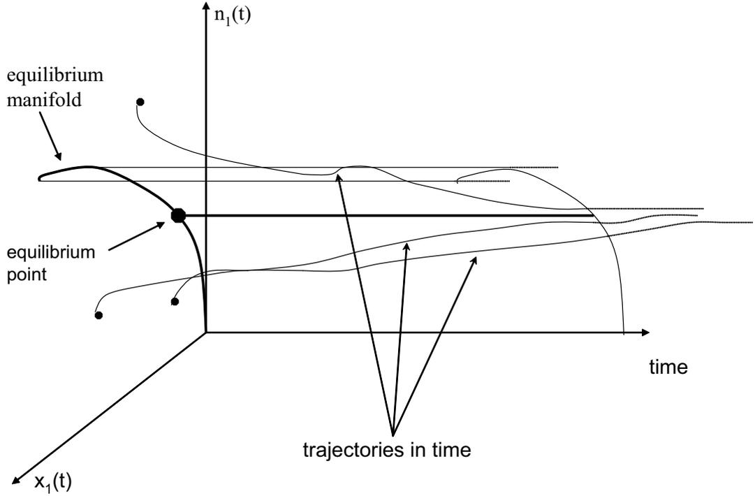
Figure 3.3. Time dynamics of a singular perturbation system.
