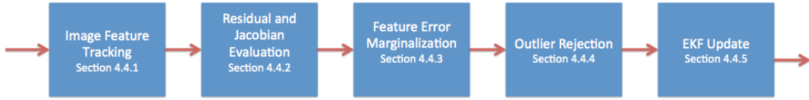
Figure 4.2: The flowchart for the camera data fusion algorithm.
