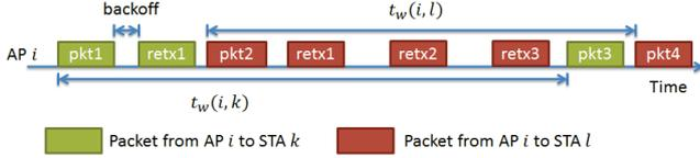
Figure 2. Illustration of  $t_w(i, k)$ .
