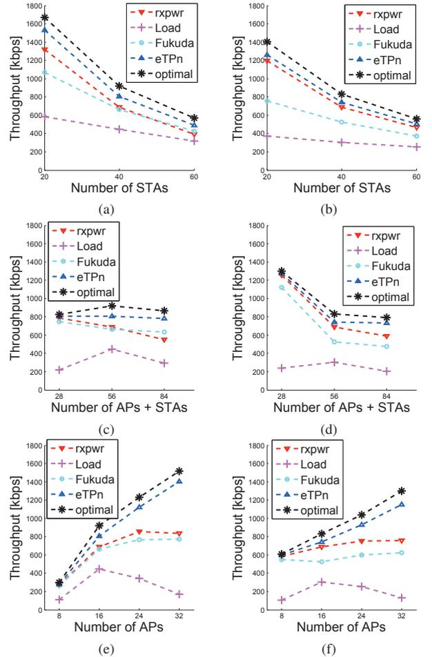
Figure 3. Average throughput of the joining STA achieved by different AP selection algorithms as a function of: (a) UDP traffic: STA density with 16 APs; (b) TCP traffic: STA density with 16 APs; (c) UDP traffic: total node density with STA to AP ratio fixed at 5:2; (d) TCP traffic: total node density with STA to AP ratio fixed at 5:2; (e) UDP traffic: AP density with 40 STAs; (f) TCP traffic: AP density with 40 STAs.
