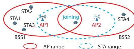
Figure 1. APs with Overlapping BSSs.
