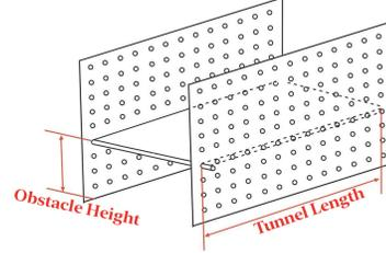
Fig. 5: Physical design of a squeezing environment.
