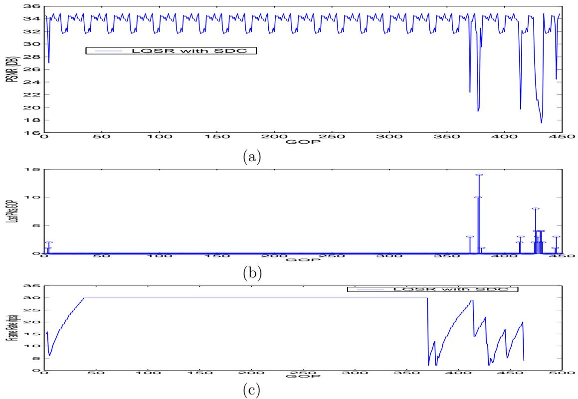
Figure 1.5: Performance Evaluation of LQSR/SDC over 802.11a (a) PSNR of the received frames; (b) Lost frames per GOP for the stream; (c) Sending frame rate.
