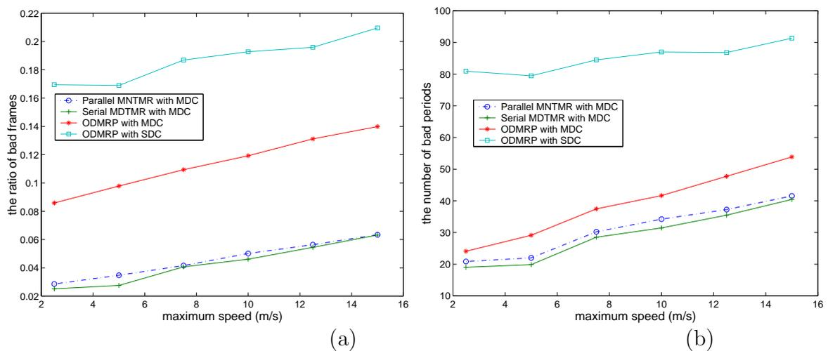
Figure 1.9: Performance evaluation for multiple tree video multicast: (a) The ratio of bad frames; (b) The number of bad periods.
