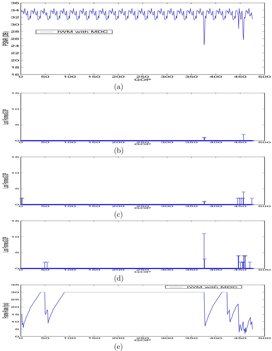
Figure 1.4: Performance Evaluation of IWM/MDC over 802.11a (a) PSNR of the received frames; (b) Number of Frames lost in both descriptions; (c) Lost frames per GOP for substream 0; (d) Lost frames per GOP for substream 1; (e) Sending frame rate.
