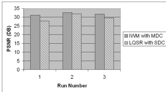
Figure 1.7: PSNR performance evaluation of IWM/MDC for 802.11a with moving nodes.
