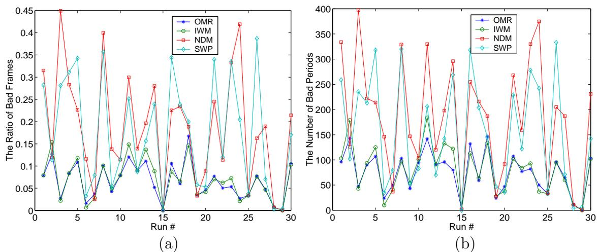
Figure 1.1: Simulation Results for the  $7 \times 7$  grid network: (a) The ratio of bad frames; (b) The number of bad periods.
