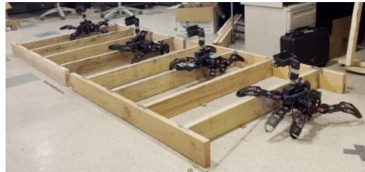
(b) Time-lapse photo of SpiderPi climbing over joists
